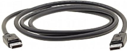
C-DP is a high-resolution DisplayPort cable for video signals up to 4K@60Hz (4:4:4) resolution supporting DisplayPort 1.2 standard. C-DP supports an HBR2 (High Bit Rate 2) bandwidth of up to 21.6 Gbps. The cable is triple shielded for superior noise immunity
